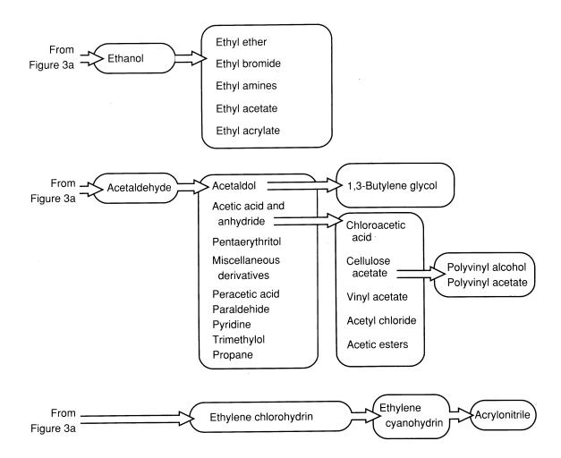
Figure 3c Important derivatives of ethylene (continued)
