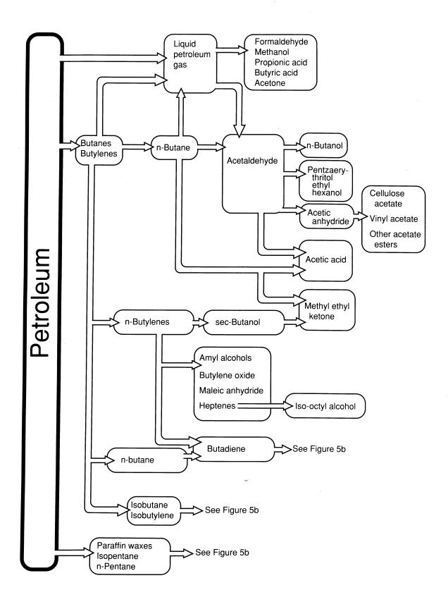
Figure 5b Important derivatives of butanes, butylenes, Liquid Petroleum Gas (LPG) and higher aliphatic hydrocarbons (continued)
