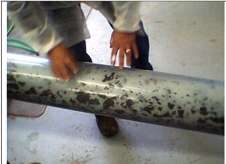
Figure 6. Gravel in column is encapsulated with pHoam™ after feed was suspended
